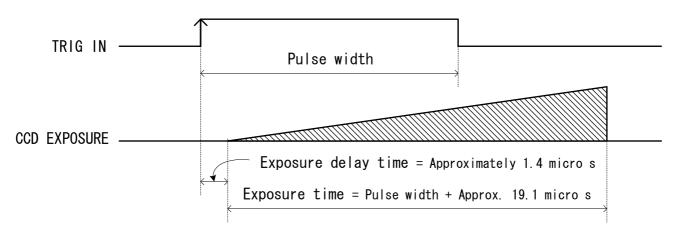
(a) Non-reset mode (Under internal sync / external sync --- Consecutive VD IN) Exposure starts at the timing of TRIG signal IN. After each exposure is completed, the camera outputs video at each next VD IN timing.
