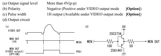
(2) HD·VD pulse (Switching via internal SW / Initial factory setting: Input)
