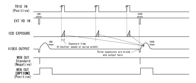
(5-4) Restart / Reset------The restart / reset function is available with the ext.VD signal.
