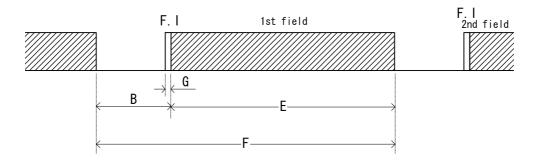
Digital output: Field ID signal superposed 1 line ahead of VS
