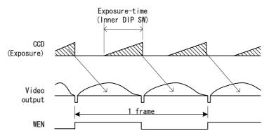
(2) Under random trigger shutter operation (Frame output)
